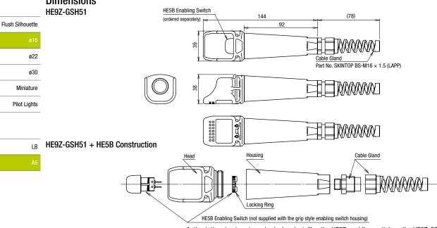
• Anti-rotation ring is not required when installing the HE5B enabling switch on the HE9Z-GSH51 grip style enabling switch housing. Use the locking ring only.
