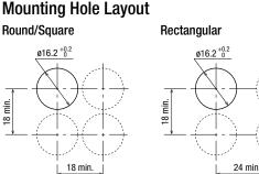
Note: Determine mounting centers to ensure easy operation.
