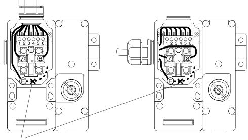
Note: When wiring the ground (E) terminal, connect in the solid line direction only. Do not connect in the dotted line direction.
