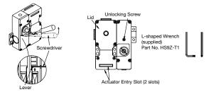
Note: Before manually unlocking the interlock switch, make sure that the machine has come to a complete stop. Manual unlocking during operation may unlock the interlock switch before the machine stops, and the function of interlock switch with solenoid is lost. After unlocking, ensure to install the screw.
