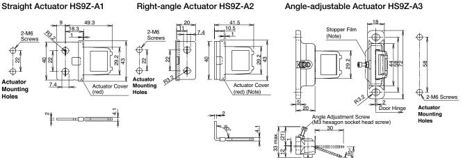
Note: The actuator cover and actuator stop films are supplied with the actuator and used when adjusting the actuator position. Remove the actuator cover and actuator stop film after the actuator position is determined.
