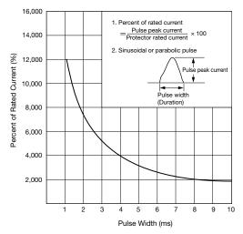
Note: Inertia delay is designed not to trip on a pulse of 20 times the rated current (peak value) for a duration of 8 ms. See the above curve.
