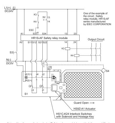
Use the monitoring device(Safety relay module) provided the capability to detect a cross short circuit. The insulation of the cable has to withstand environmental influences. If a control device other than the one shown in the draft is used, the used control device has to be equipped with a cross short circuit monitor
